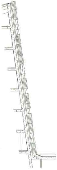
Detail section through exterior stone wall | 10'
